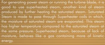
To run turbine blades the steam needs to be having more of a kinetic energy and must be free from moisture as moisture is undesirable with moving parts. Superheated steam is therefore the best medium to run turbine and generate electricity.
